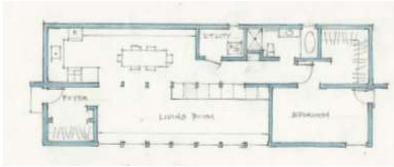
This sample floor plan illustrates a 1040 square feet (20' x 52'), 1 bedroom plan with generous living spaces. Any size from 240 square feet on up can be built. Every plan is custom designed to meet your spatial and building site requirements. All construction plans are engineer certified and
