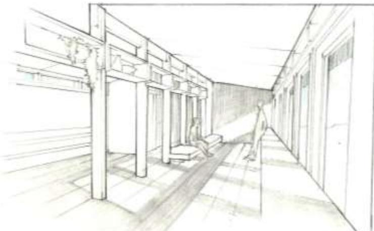
Structural clerestory windows, providing even natural lighting, is incorporated into this model which supports the roof, so there is no need for the timber trusses of the original Noble Home kit. Additionally, a series of wood interior ridge support units help divide the space while adding storage and providing a structural and aesthetic richness to the space. Additional storage and/or seating options can be fixed to these units in more compact homes.
